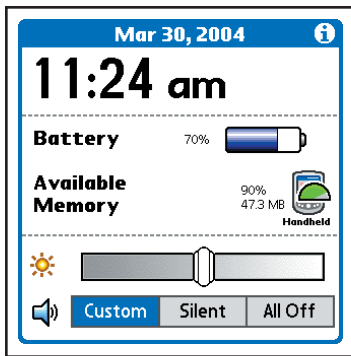
Figure B.24 Tapping the System Information button gives you battery and memory statistics as well as controls for audio and screen brightness.
